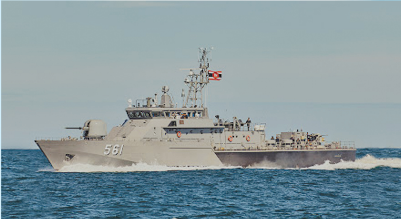
Royal Thai Navy 58m@27knots Large Patrol Craft built by Marsun Shipyard submitted to Bangladesh Navy Tender as a proven vessel.
